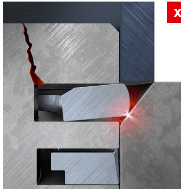
Fig. 1: Chamfer on the cylinder bore too large – the piston rebounds between the piston ring scuff band and cylinder during mounting and the piston becomes blocked
