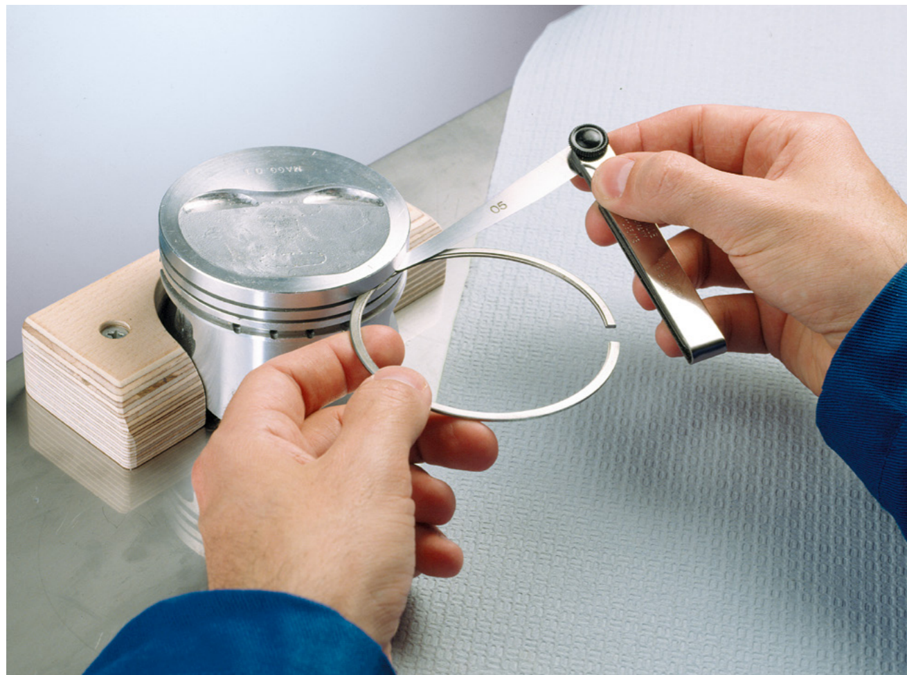
Fig. 1: Measuring the ring height clearance
