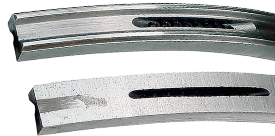
Fig. 3: New and worn oil control ring
