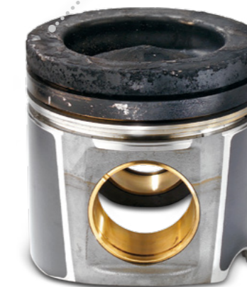
Fig. 3: Carbon layer on the top land
