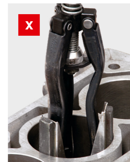
Fig. 2: Spring-loaded honing stones
