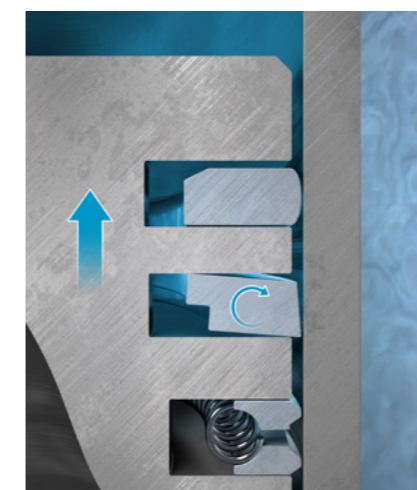
Fig. 5: Without combustion pressure
