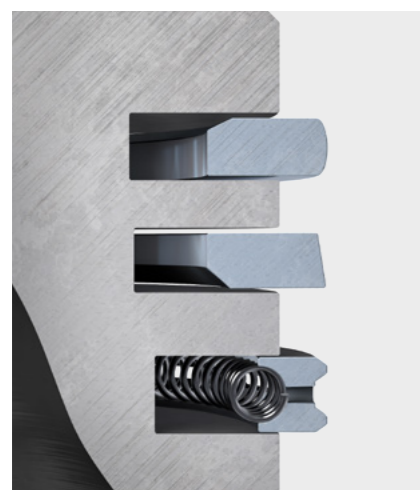
Fig. 2: Piston rings untensioned – twisting still ineffective
