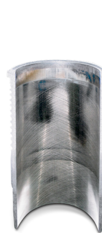
Fig. 2: Bright and polished areas in the top cylinder area
