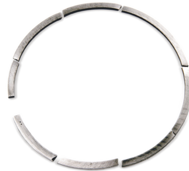
Broken piston ring
