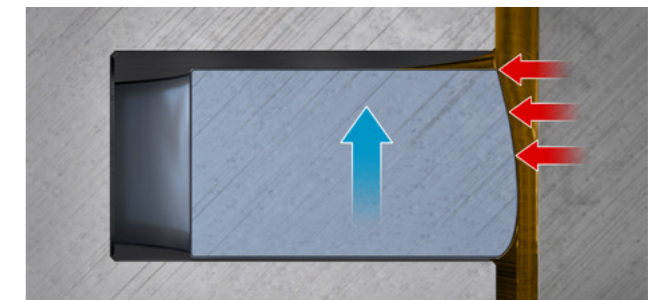
Fig. 4: High floating during the upwards movement
