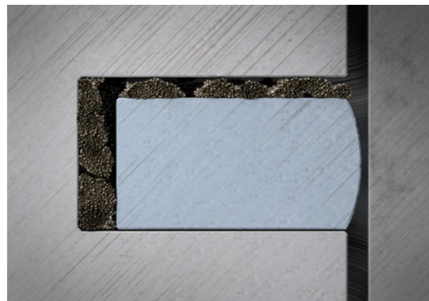
Fig. 1: Dirt deposit in the ring groove
