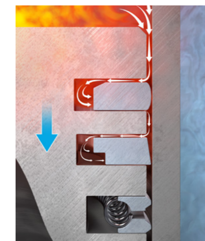
Fig. 6: With combustion pressure
