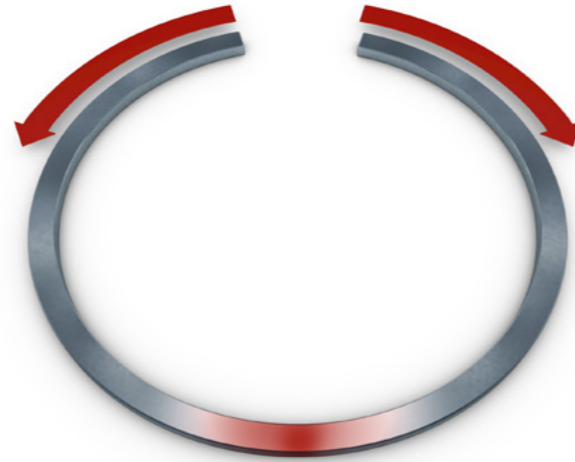
Fig. 1: Excessive spreading of the piston ring
