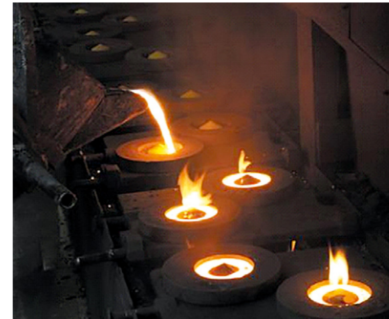
Piston ring casting process
